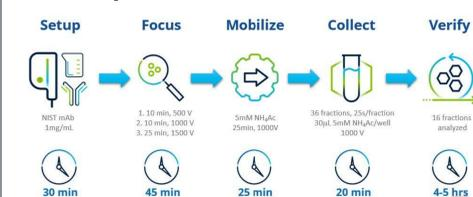
icIEF fractionation was carried out on a MauriceFlex system (Bio-Techne) on NISTmAb samples. The charge fractions were verified for identity and purity before being pooled for peptide mapping analysis on a High-Resolution Mass Spectrometer (Thermo Fisher).
