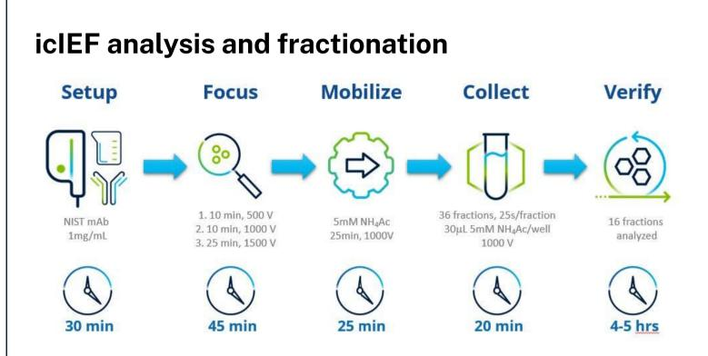
icIEF fractionation was carried out on a MauriceFlex system (Bio-Techne) on NISTmAb samples. The charge fractions were verified for dentity and purity before being pooled for peptide mapping analysis on a High-Resolution Mass Spectrometer (Thermo Fisher)
